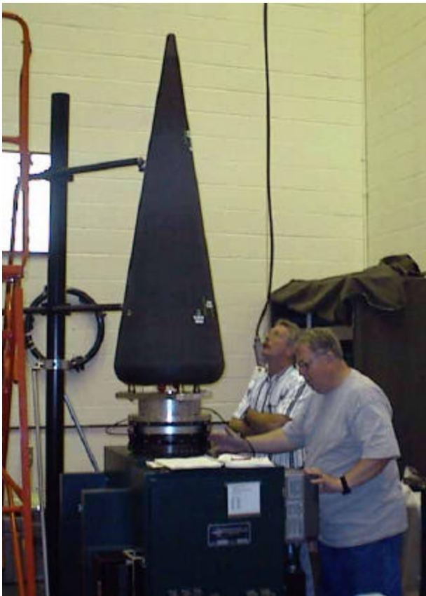
Figure 7 Using two dial indicators to adjust tilt
