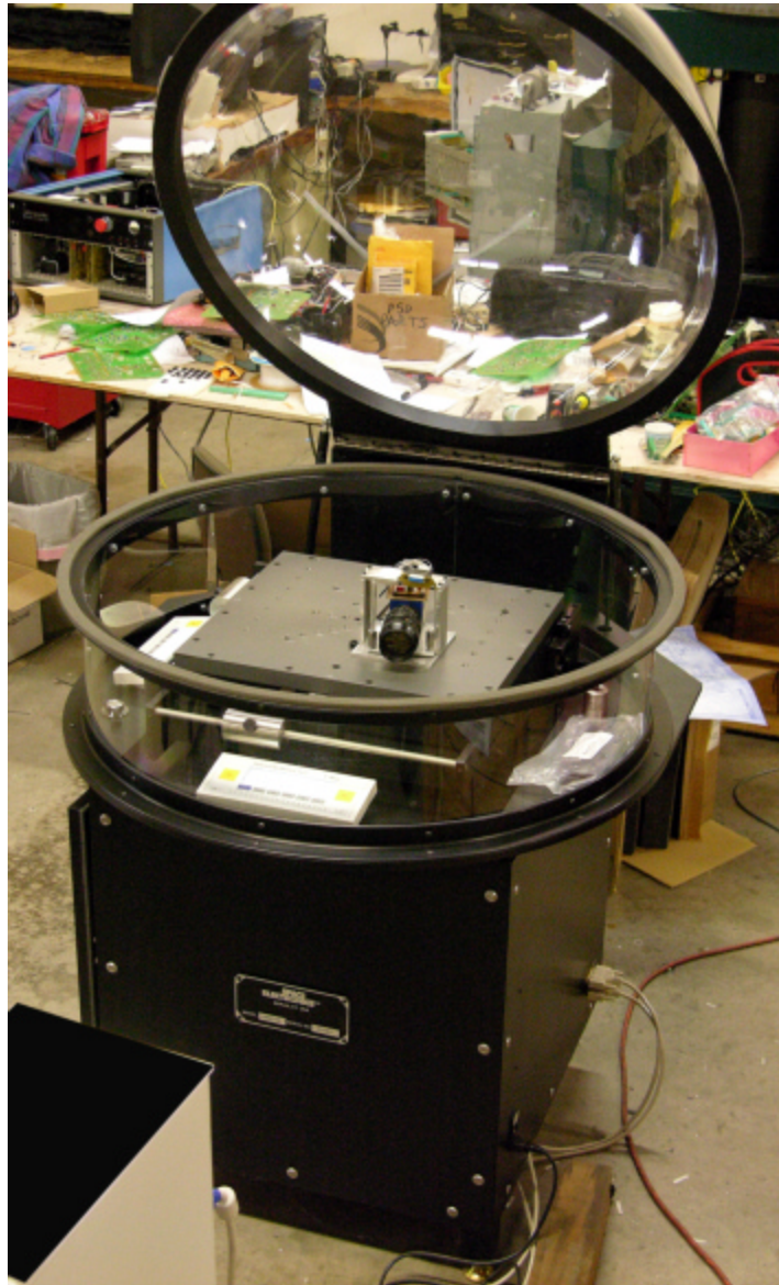
Figure 8. Gimbaled Camera Assembly on balance machine
