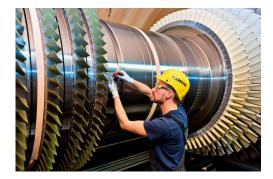
Unbalance within turbine machinery spinning at >3000 RPM will result in fluctuating power output as well as unreliability and damage over time. Static balancing of rotor stages and individual blades will alleviate these issues and provide you with reduced operational costs.
