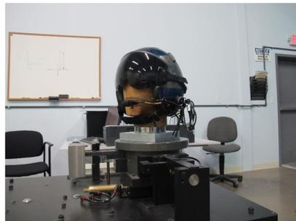
Raptor Scientific offers products and services to measure Weight, Center of Gravity, Moment of Inertia, and Product of Inertia for a wide range of objects such as helmets, golf balls and clubs, steering wheels, drive shafts, medical tools, disc drive heads, drones, propellers, electronic circuit boxes, and many other objects.
