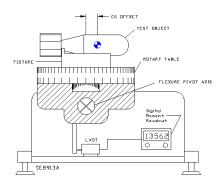
A rotary table is mounted on a precision spindle bearing. Crossed web flexures provide a horizontal pivot axis which is essentially frictionless. A torsion rod in line with this pivot axis creates a linear torsion spring about this axis. When the test part CG is displaced from the measurement axis, an unbalance moment is created, resulting in a displacement of the LVDT mounted at the end of the moment arm.
