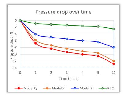
**Conclusion:** The metal capillary hose pressure loss was noticeably less than the synthetic hoses by at least a factor 4.
