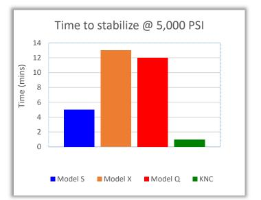
Conclusion: The metal capillary hose stabilized almost immediately, the synthetic hoses took up to 13 minutes to stabilize.
