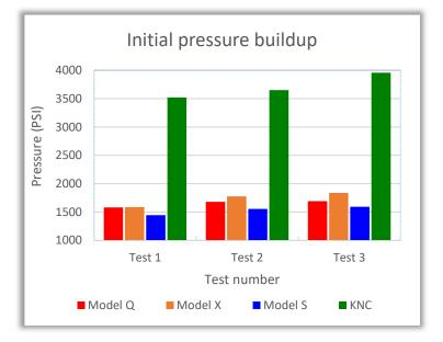
**Conclusion**: Not surprisingly a hose with smaller ID and lower overall volume allows for a significantly higher pressure generation using the same pump stroke.
